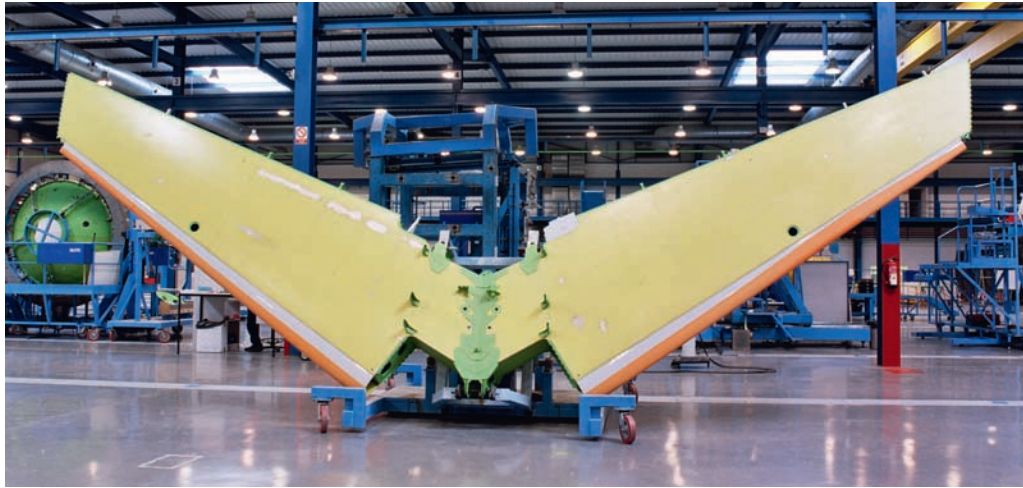
HEGAN member company, Aernnova : Responsible for the design and manufacture of structures for the Airbus A350 XWB horizontal tail plane and elevator
