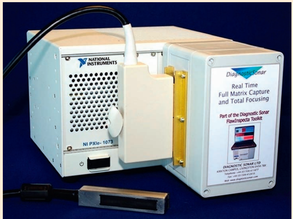
Diagnostic Sonar's FlawInspecta: Uses two PXI slots for full matrix capture and total focusing at real-time rates
